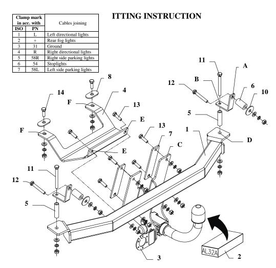
This towing hitch is designed to assembly in following car: **ALFA ROMEO 146, 5 doors,** produced since 1995 till 2001, catalogue no. **AL32A** and is prepared to tow trailers max total weight **1300 kg** and max vertical load **75 kg**.
