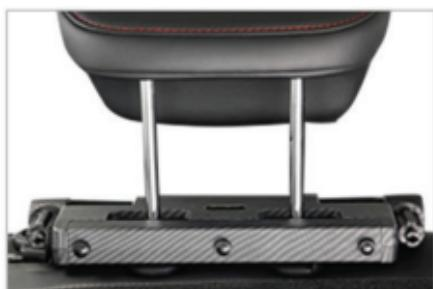
2. Adjust the sliding rod to a suitable position and install it on the headrest rod, cover the back cover and tighten the 3 screws by hand.
