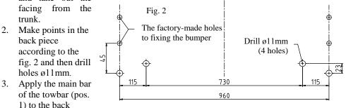
piece and fix through made holes and the washers (pos. 9) using bolts M110x30mm (pos. 8) from the accessories.
