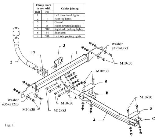
This towbar is designed to assembly in following cars: **AUDI 80, 4 doors, except Quattro, (B3),** produced since 09.1986 till 08.1991, catalogue no. **A16** and is prepared to tow trailers max total weight **1500 kg** and max vertical load **50 kg**.
