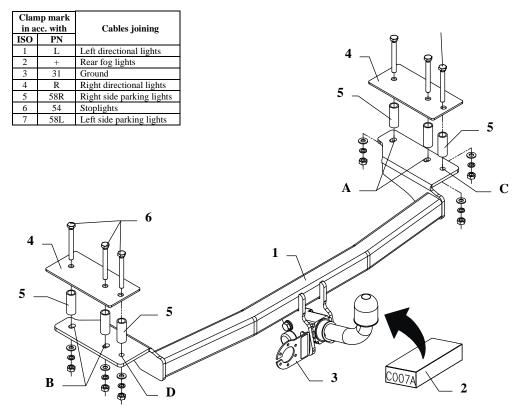
This towbar is designed to assembly in following cars: **FORD ESCORT I, 3/5 door,** produced since 01.1986 till 09.1990, catalogue no. **C007A** and is prepared to tow trailers max total weight **1200 kg** and max vertical mass **50 kg**.
