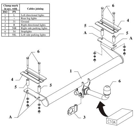
This towing hitch is designed to assembly in following cars: **FORD ESCORT, 3/5 doors, Cabrio, except 4x4,** produced since 01.1996 till 10.1998, catalogue no. **C10A** and is prepared to tow trailers max total weight **1250 kg** and max vertical mass **50 kg**.
