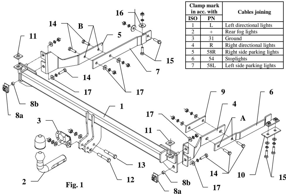
This towbar is designed to assembly in following cars: **MERCEDES 190, 4 doors (W201)**, produced since 10.1982 till 09.1988, catalogue no. **D04** and is prepared to tow trailers max total weight **1500 kg** and max vertical load **75 kg**.
