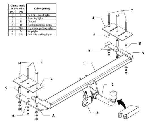
This towing hitch is designed to assembly in following car: **OPEL VECTRA (A), 4 doors, except 4x4,** produced since 09.1988 till 08.1995, catalogue no. **E11A** and is prepared to tow trailers max total weight **1700 kg** and max vertical load **75 kg**.
