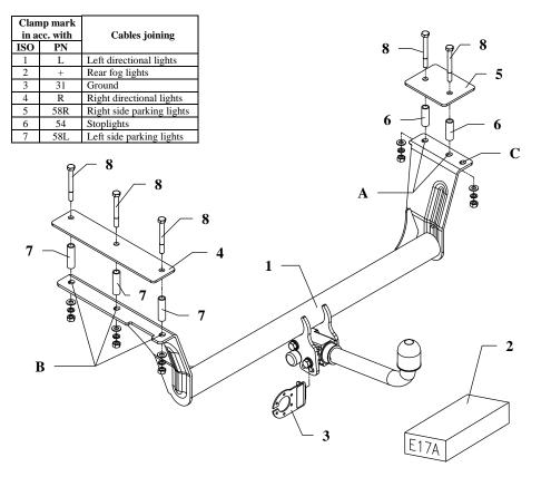
This towbar is designed to assembly in following cars: **OPEL OMEGA B Caravan, ESTATE,** produced since 04.1994 till 07.2003, catalogue no. **E17A** and is prepared to tow trailers max total weight **2100kg** and max vertical load **75kg**.
