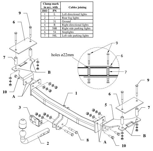
This towing hitch is designed to assembly in following car: **OPEL COMBO (B), passenger car, delivery truck,** produced since 08.1995 till 02.2002, catalogue number **E20** and is prepared to tow trailers max total weight **1200 kg** and max vertical load **50 kg**.
