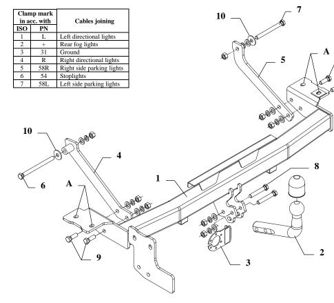
This towbar is designed to assembly in following car: **HYUNDAI H200; SATELITE/STAREX (H1) VAN,** produced since 01.1997 till 01.2008, catalogue no. **J15** and is prepared to tow trailers max total weight **2000 kg** and max vertical load **80 kg**.
