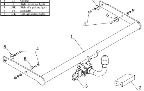
The towbar can be used in the following car: VOLKSWAGEN GOLF III VARIANT, ESTATE, 4x4, produced since 10.1993 till 07.1999, catalogue number K16A and is prepared to tow trailers max total weight 1500 kg and max vertical load 75 kg
