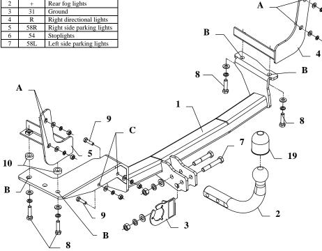
This towbar is designed to assembly in following car: VOLKSWAGEN POLO 3/5 door (6N1), produced since 09.1994 till 09.1999, catalogue no. **K21** and is prepared to tow trailers max total weight 1400 kg and max vertical load 50 kg.
