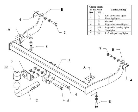
This towing hitch is designed to assembly in following cars: **VOLKSWAGEN CADDY passenger car/delivery van**, produced since 11.1995 till 01.2004 **SEAT INCA passenger car/delivery van** produced since 11.1995 till 06.2003, catalogue no. **K31** and is prepared to tow trailers max total weight **1100kg** and max vertical load **50 kg**.
