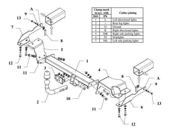
This towing hitch is designed to assembly in following cars: **TOYOTA YARIS**, 3/5 doors, (CP10), except TS, Japanese and French version, produced since 04.1999 till 12.2005, catalogue no. O24 and is prepared to tow trailers max total weight 900 kg and max vertical load 50 kg.
