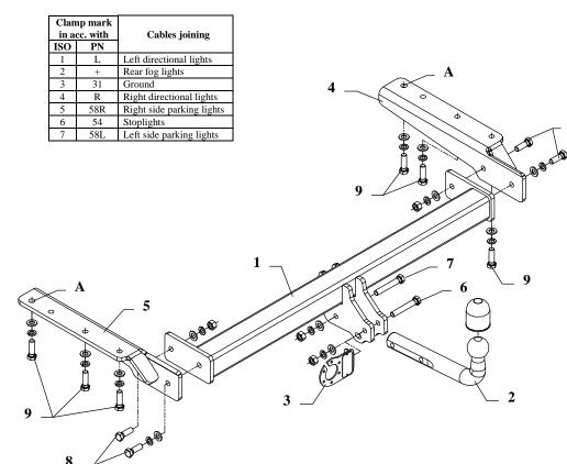
This towbar is designed to assembly in following cars: **TOYOTA LANDCRUISER J90/J95, 3 door,** produced since 04.1996 till 12.2002, catalogue no. **O45** and is prepared to tow trailers max total weight **3500 kg** and max vertical load **140 kg**.
