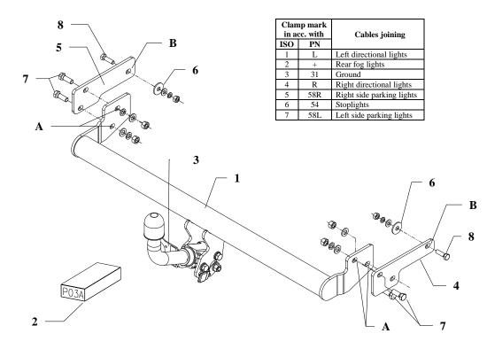
This towbar is designed to assembly in following car: CITROEN ZX 3/5 DOORS (N2), produced since 03.1991 till 06.1997, catalogue number P03A, and is prepared to tow trailers max total weight 1100 kg and max vertical load 70 kg.
