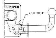
4. To the chassis of car put main bar of the towbar (pos. A) and through holes pos. 2 and 3 fix with already mounted side brackets (pos. C) using bolts M10x45mm.
