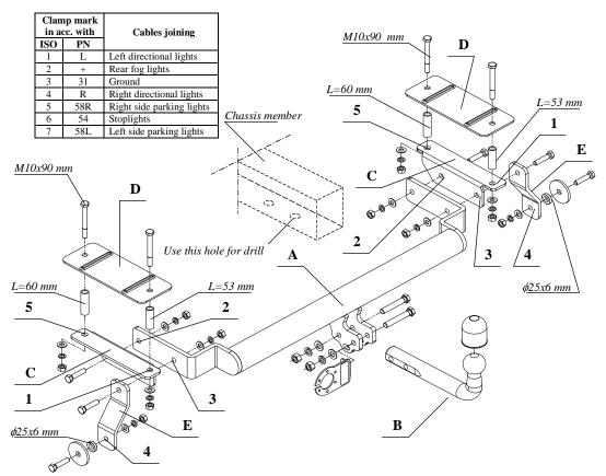
This towing hitch is designed to assembly in following car:
