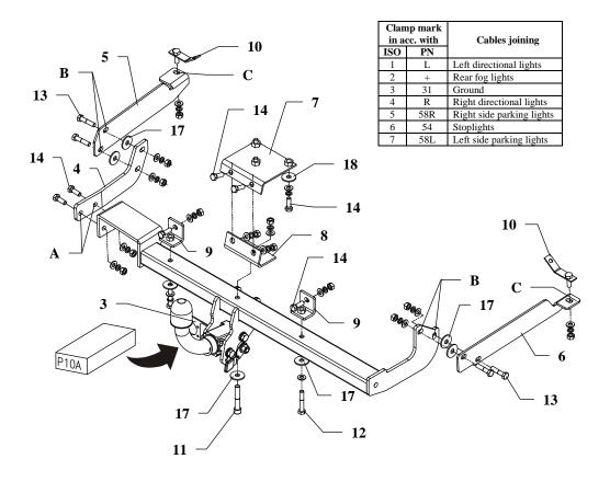
This towbar is designed to assembly in following cars: CITROEN XSARA, 3/5 doors (N1), produced since 04.1997 till 03.2005, catalogue no. P10A and is prepared to tow trailers max total weight 1300 kg and max vertical load 70 kg.
