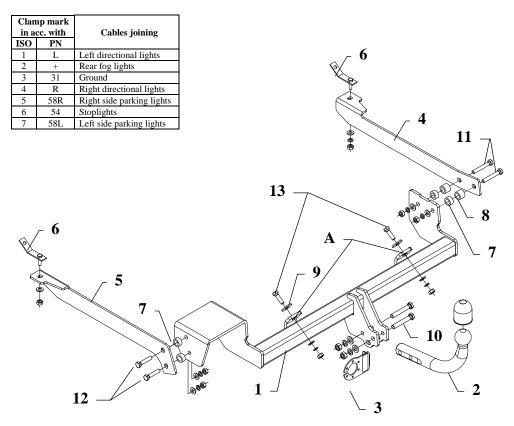
This towing hitch is designed to assembly in following cars: CITROEN XSARA Break, ESTATE (N2), produced since 01.1997 till 03.2005, catalogue no. P14 and is prepared to tow trailers max total weight 1300 kg and max vertical load 80 kg.
