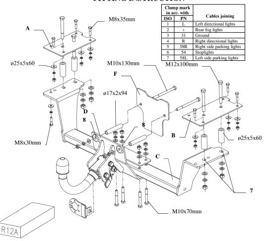
This towbar is designed to assembly in following car: **FIAT MAREA WEEKEND ESTALE** (185), produced since 10.1996 till 10.2002, catalogue no. **R12A** and is prepared to tow trailers max total weight 1400 kg and max vertical load 70 kg.
