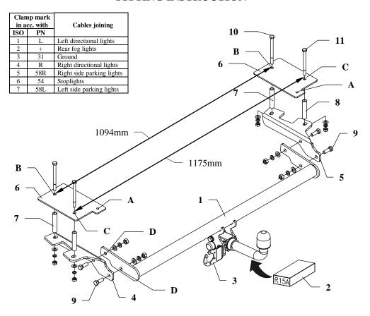
This towing hitch is designed to assembly in following cars: **FIAT PALIO WEEKEND ESTATE** (178), produced since 01.1998 till 10.2003, catalogue no. **R15A** and is prepared to tow trailers max total weight 1200 kg and max vertical mass 70 kg.
