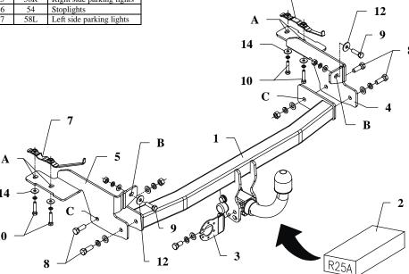
This towbar is designed to assembly in following cars: **FIAT PUNTO II, 3/5 doors VAN (188), except Sport,** produced since 09.1999 till 2011, catalogue no. **R25A** and is prepared to tow trailers max total weight **1400 kg** and max vertical mass **75 kg**.
