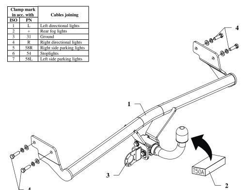
This towbar is designed to assembly in following cars: **KIA RIO, 5 doors,** produced since 08.2005 till 09.2009, catalogue no. **T50A** and is prepared to tow trailers max total weight **1100 kg** and max vertical load **50 kg**.
