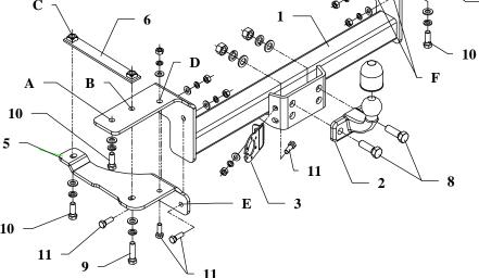
This towing hitch is designed to assembly in following cars: **SUZUKI SAMURAI**, 3/5 doors, produced since 1982, catalogue number **W06** and is prepared to tow trailers max total weight up to **1300 kg** and max vertical mass **75 kg**.
