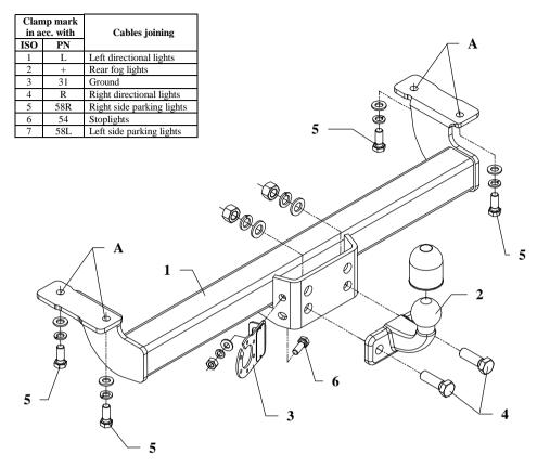
This towing hitch is designed to assembly in following cars: **SUZUKI VITARA, 3 doors, except V6,** produced since 10.1988 till 08.1998, catalogue no. **W07** and is prepared to tow trailers max total weight **1500 kg** and max vertical mass **75 kg**.
