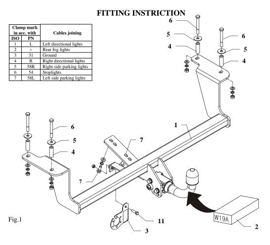
This towing hitch is designed to assembly in following car: **SUZUKI IGNIS II, 3/5 doors, 2/4WD** produced since 09.2003 (in Hungary), catalogue no. **W19A** and is prepared to tow trailers max total weight **800** kg and max vertical load **50** kg.
