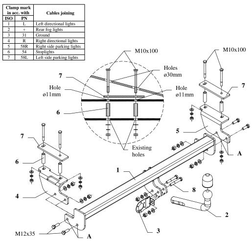
This towbar is designed to assembly in following cars: **DAEWOO NEXIA, 3-5 door,** produced since 02.1995 till 08.1997, catalogue no. **X02** and is prepared to tow trailers max total weight **1200 kg** and max vertical load **70 kg**.
