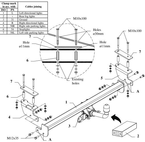
This towbar is designed to assembly in following cars: **DAEWOO NEXIA, 3-5 door,** produced since 02.1995 till 08.1997, catalogue no. **X02A** and is prepared to tow trailers max total weight **1200 kg** and max vertical load **70 kg**.
