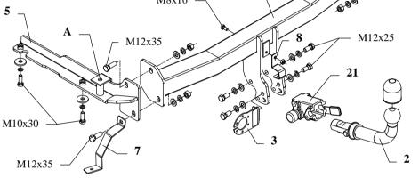
This towbar is designed to assembly in following cars: **DAEWOO NUBIRA II, 4 door,** produced since 07.1999 till 2003, catalogue no. **X11A** and is prepared to tow trailers max total weight **1200 kg** and max vertical load **70 kg**.
