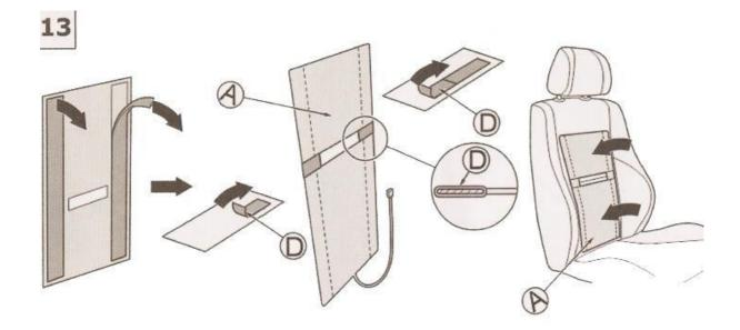
The electrodes on the ends of rectangle aperture (s) must be enwrapped with doubt coated adhesive protection tape Fig 7\_1 and D.
