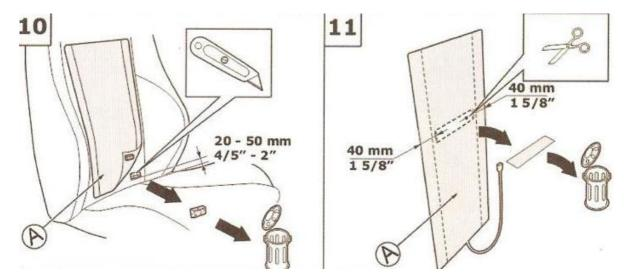
The foam opposite to the temperature controller should be cut into a hole, in order to level the pad. If there are fillisters for trimming wires on the seat or backrest, the heating area of pad within the two electrode tapes should be delineated with pencil or marker pen and cut into a rectangle aperture with 40mm width as illustrated in **11**.
