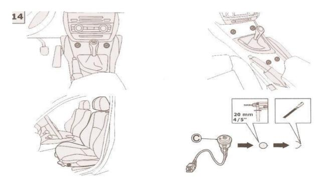
At the proper position such as near gear-level, flanks of the seat, auxiliary fascia console, etc. a hole is drilled to install the switch. The fillisters for reinforcing ribs of the switch should be filed.
