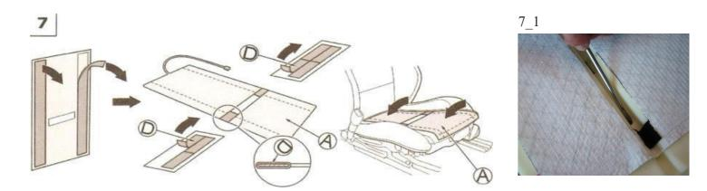
The electrodes on the ends of rectangle aperture (s) must be enwrapped with doubt coated adhesive protection tape Fig 7\_1 and D. The backing should be ripped when the pads are installed.
