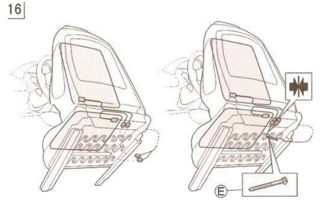
The harness connecting with seat pad and backrest pad is distributed as above. The harness should be bound with Nylon cable tie  $\circ$
