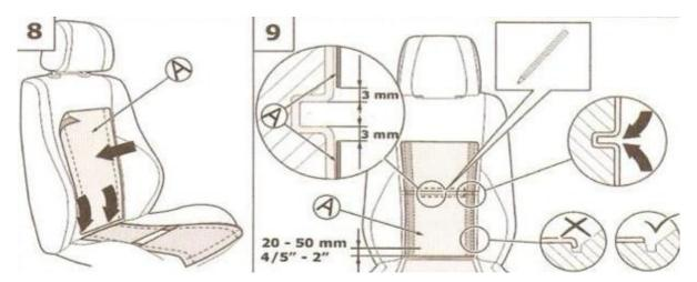
The backrest of heating pad should be unfold as illustrated in **8** The installation of the backrest on the fillisters is the same as **2** & **4**. There are at least 3mm between the pad and fillisters after the pad is unfolded nicely. The heating area can not be put inside of any fillisters.
