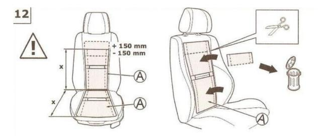
There are  $\pm 150$ mm cutting deviations of either seat or backrest. Superfluous parts of the pad must be cut off. The backing should be ripped when the pads are installed.
