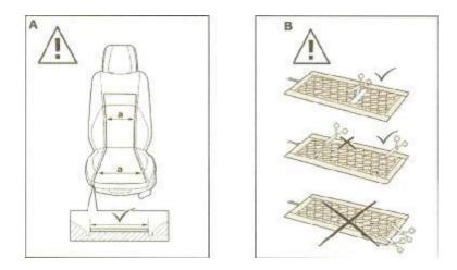
Refer to the safety instructions for handling airbag modules and pyrotechnical belt tensioners. Incorrect handling may cause the pyrotechnical belt tensioner or side airbag to deploy and thus cause injuries.
