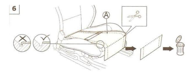
Superfluous parts of the pad must be cut off.
